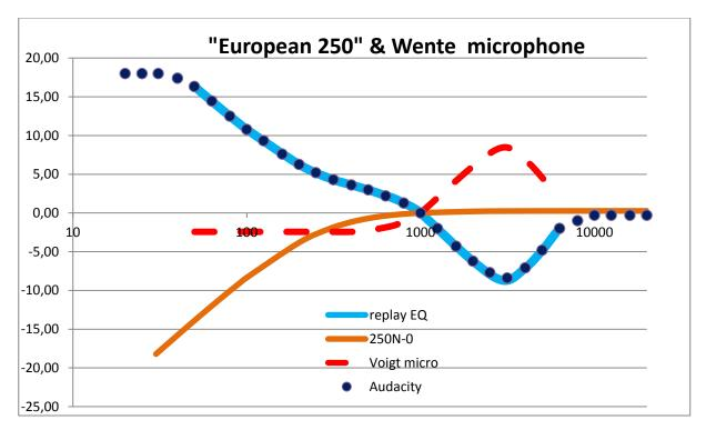
This chart shows the most likely recording curve "250N-0" in combination with a W.E. mod. 361 microphone as described by Voigt and the corresponding playback EQ.
